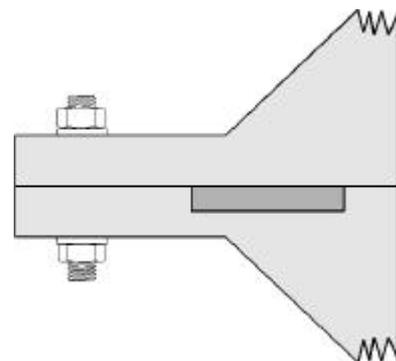
**Ring joint flange** arrangement (also known as **API Ring**), in which both flanges have channels to accept the ring joint gasket, which is usually made of solid metal. The gaskets involved are often referred to as **RTJ** or **ring type joint** gaskets:
