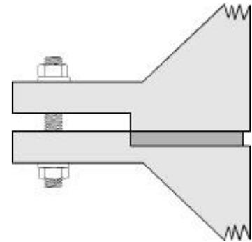
**Flat face and groove flange** arrangement, with totally confined gasket. The external face of one of the flanges is plain (flat) and the other has a groove where the gasket is installed. These designs are used in applications where the distance between the flanges must be precise. When the gasket is seated, the flanges are usually in contact with each other. Only resilient gaskets should be used in this system:
