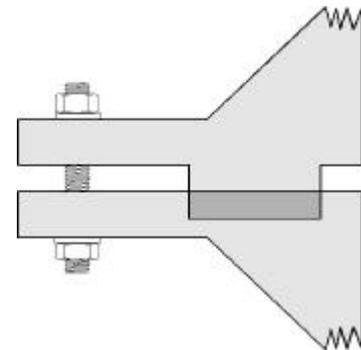
**Male and female flanges** (also known as **spigot flanges**) contain a semi-confined gasket, and may be in a variety of forms. The depth of the female flange is equal to or less than the height of the male, in order to avoid the possibility of direct contact between the flange faces when the gasket is compressed. The flange system must be separated in order to change the gasket:
