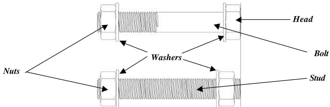
The function of the fastener is to clamp the joint sufficiently to prevent slip or leakage, and hence it must be strong enough to support the tension induced on initial tightening, together with the additional loads it will endure in service (as a result of
